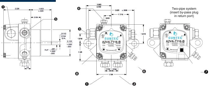
2 Return 3 Nozzle outlet 4 Pressure gauge port 5 Pressure adjustment 6 Bleeder valve
