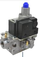
Multifunctional gas control equipped with 2 solenoid valves Class A (according to EN 161) and an outlet gas regulator (EN 88-1). Designed for pressure jet gas burners with a capacity up to 450 kW. Slow opening option available.
