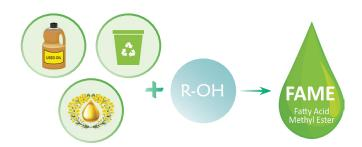
Fatty Acid Methyl Ester is a biofuel produced by a process of transesterification of biomass such as vegetable oils (rapeseed, soybean, corn, beet, etc.), animal fats, used cooking oils or greasy industrial waste.
