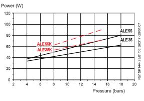
Viscosity = 5 cSt - Rated speed = 2850 rpm 1,8 cSt
