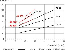
Viscosity = 5 cSt - Rated speed = 2850 rpm 1,8 cSt
