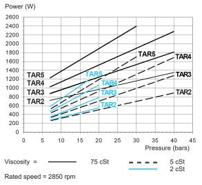
Data shown are for new pumps, with no allowance for wear.
